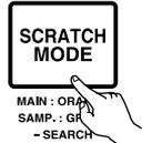
Each short push of the SCRATCH MODE button switches between MAIN and SAMPLER.
